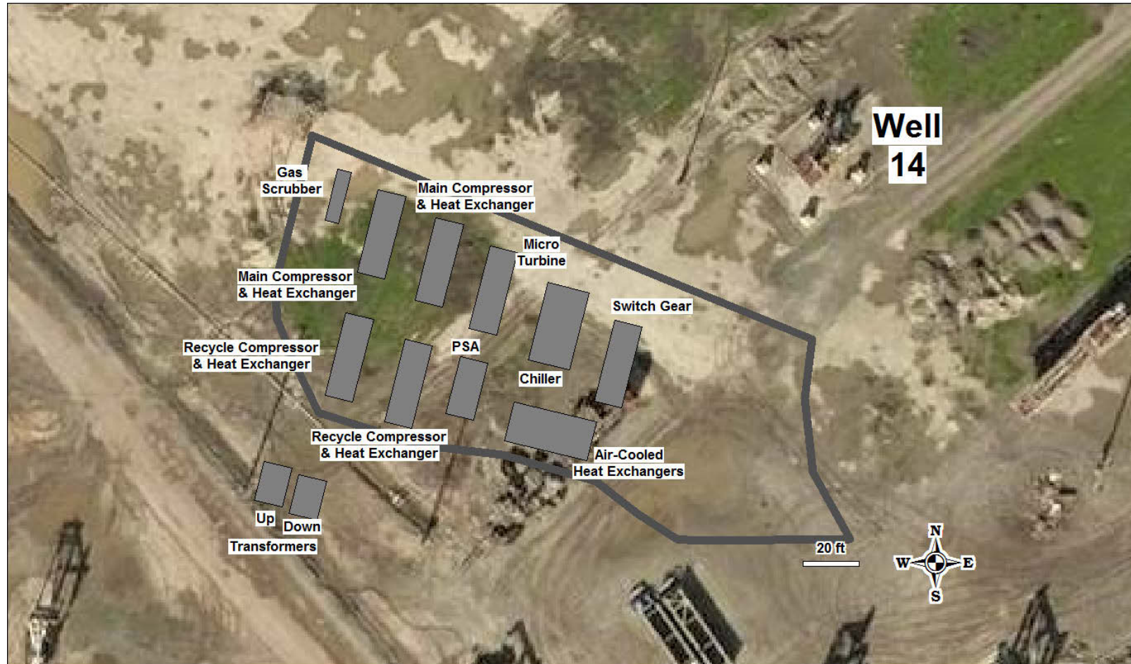
Figure 3 Equipment Layout for the Proposed Gas Plant
